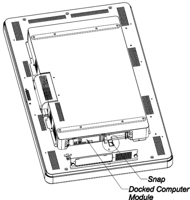
6. Replace the protective plate and tighten its thumb screws in order to mechanically secure the computer module.
