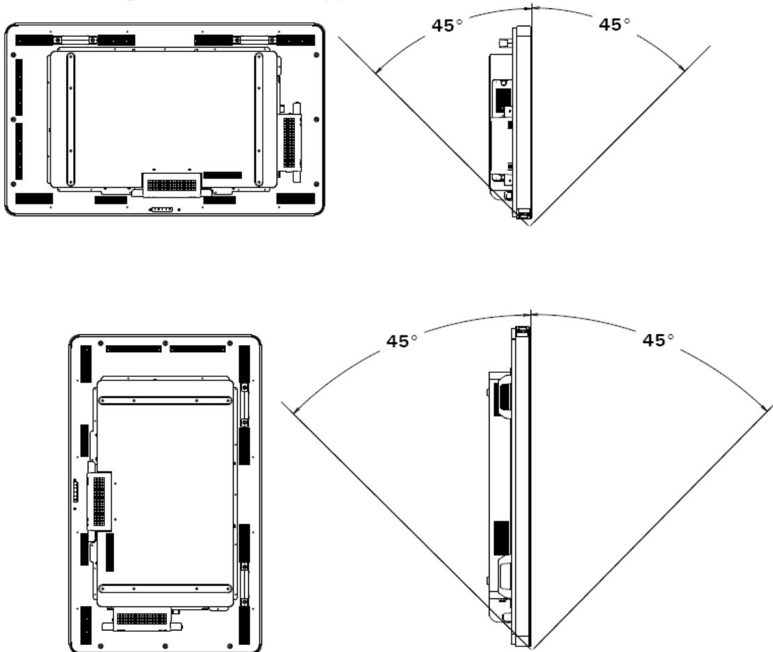
Select the desired mounting orientation from the display's On-Screen Display (OSD) Mounting menu for OSD text rotation and to change which Elo logo is lit.
