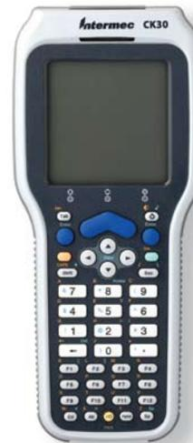
**Three distinct keypad options ranging from the simplified 42-key to a full 52-key alphanumeric offer layouts for a range of applications.**
