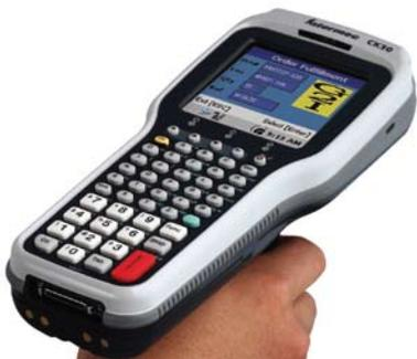
**An optional user-installable and removable pistol grip handle is ideal for highly repetitive scanning.**
